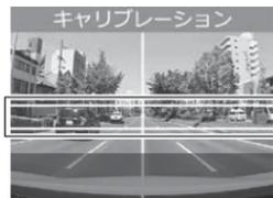
Adjust so that the horizontal lines of the road fit within the two traverse lines.
