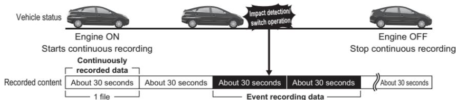
\*Saves a file on the occasion of an event (impact detection/switch operation) and two files before and after that event.
